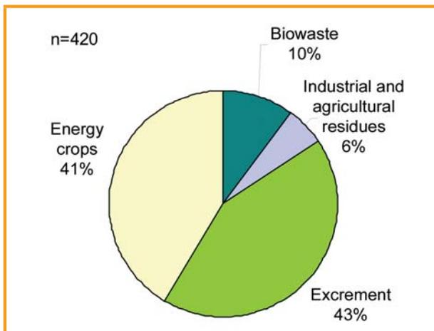
Figure 12.5: Mass-based substrate input in biogas plants (operator survey 2009) [12-3]
