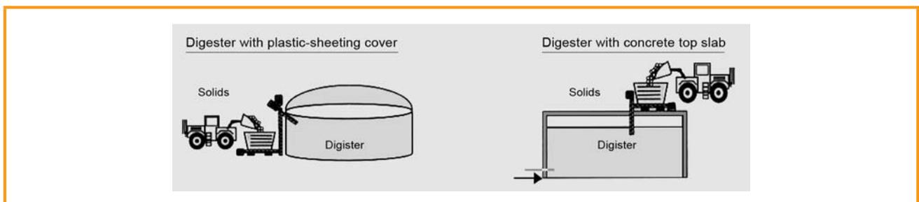
Figure 3.16: Direct solids infeed (schematic) [3-1]
