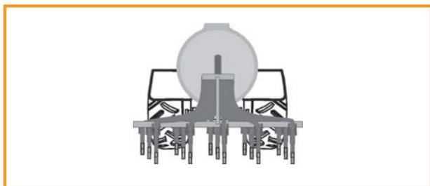
Figure 10.5: Manure injector
