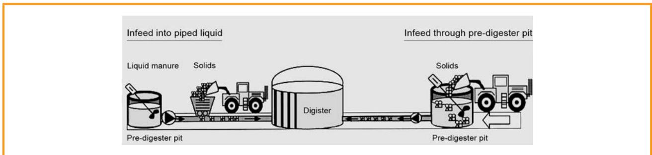
Figure 3.15: Indirect solids infeed (schematic) [3-1]
