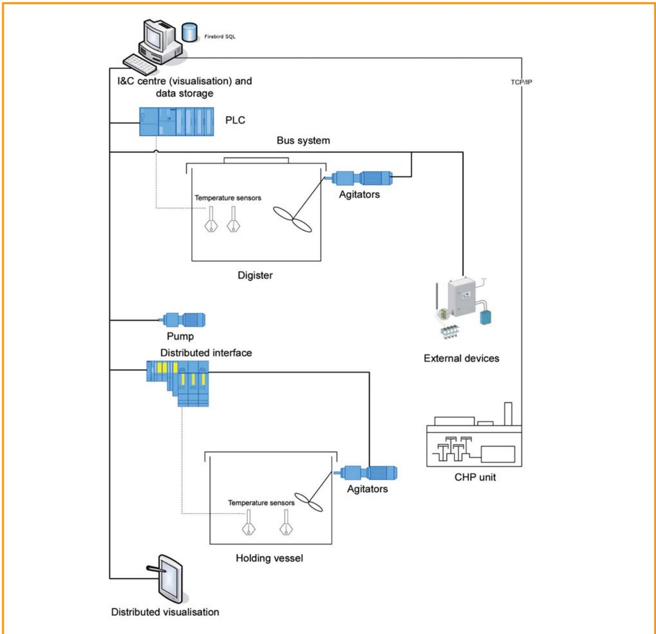
Figure 5.2: Schematic representation of plant monitoring
