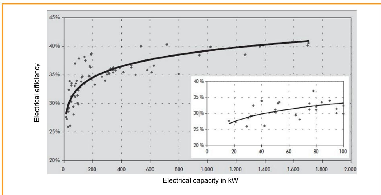
Figure 6.6: Electrical efficiency of biogas CHP units [6-41]
