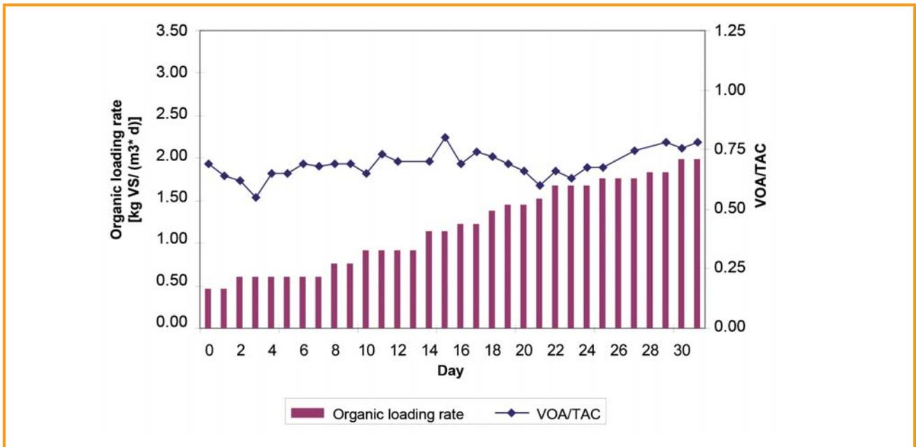
Figure 5.6: Progress of start-up phase, digester 3
