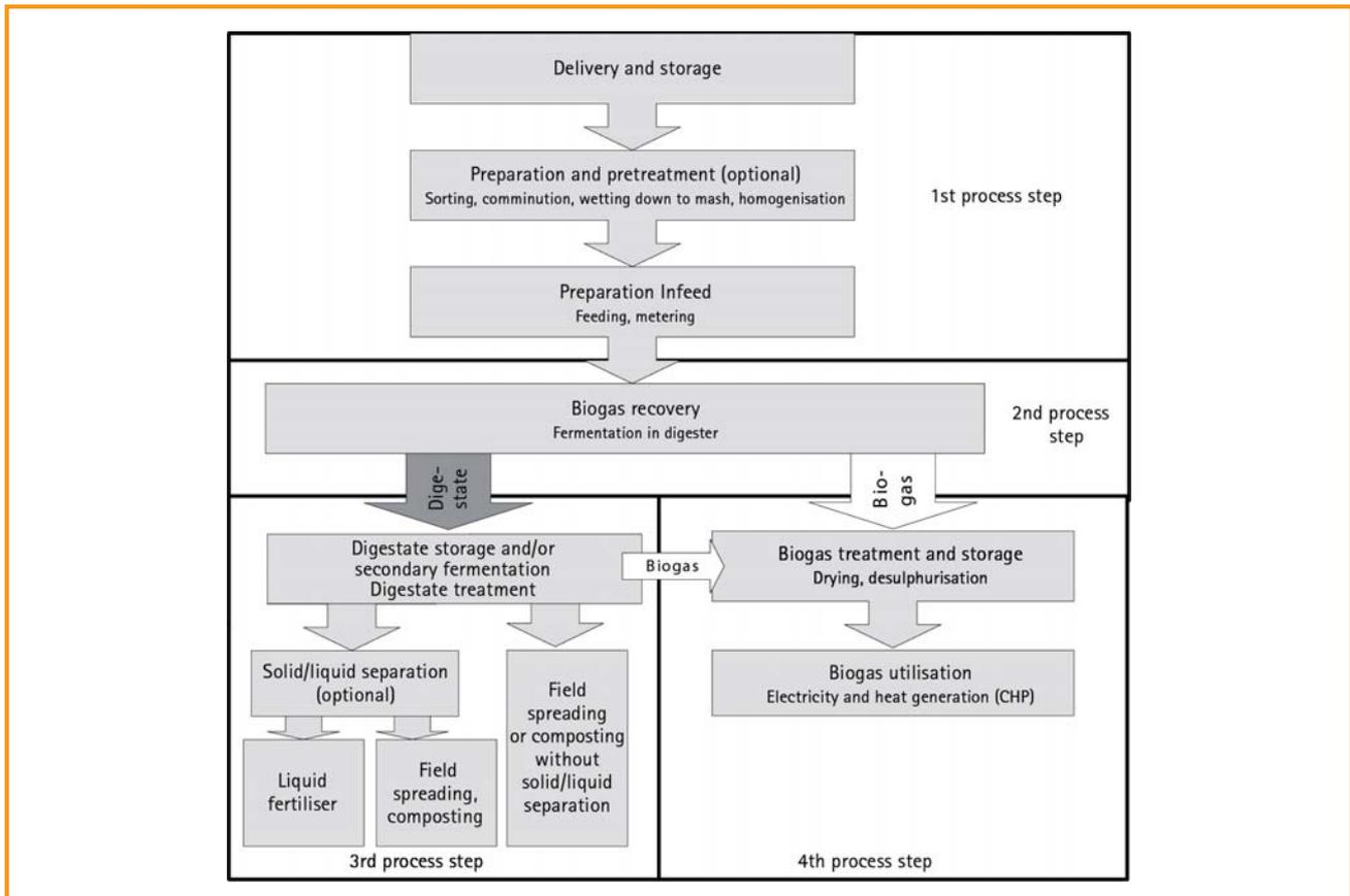
Figure 3.3: General process of biogas recovery; as described in [3-3]
