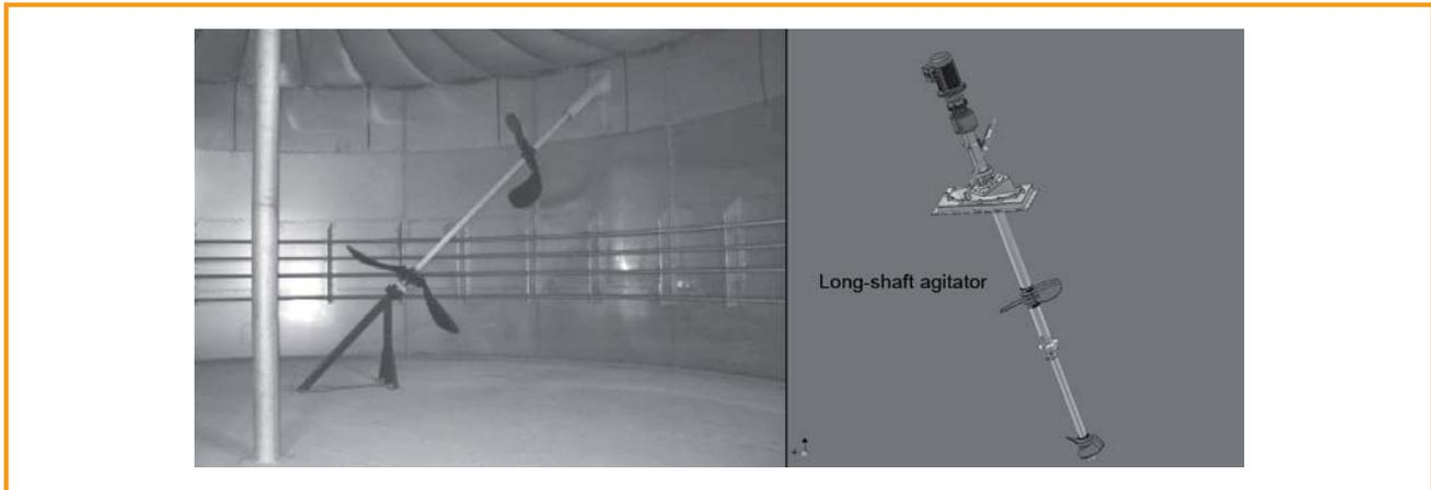
Figure 3.32: Long-shaft agitators with two stirring blades with and without shaft-end bearer on the bottom of the digester [WELtec BioPower GmbH; graphic: Armatec FTS-Armaturen GmbH & Co. KG]
