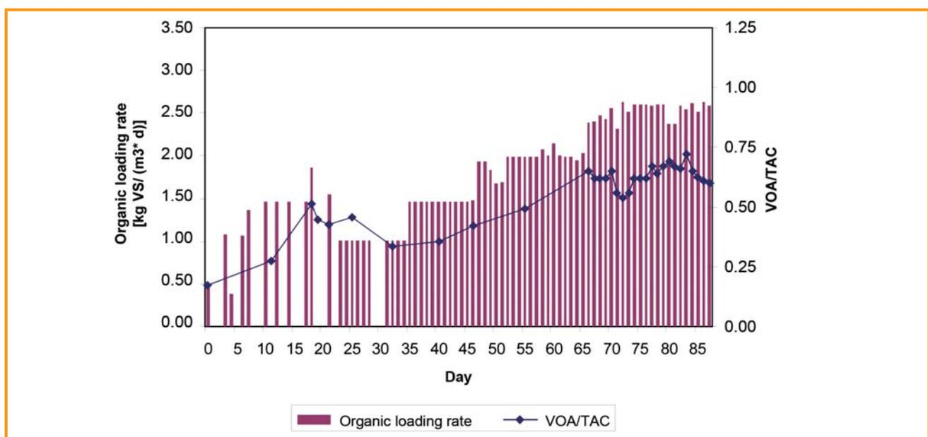
Figure 5.4: Progress of start-up phase, digester 1
