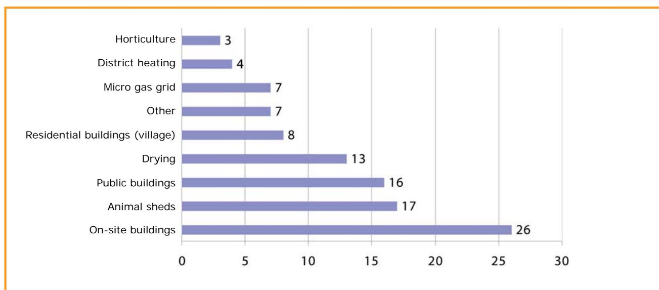
Figure 8.1: Uses of waste heat from biogas plants operating with a CHP process [8-7]
