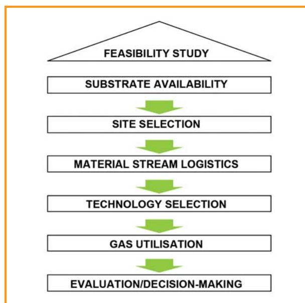
Figure 11.3: Criteria for a feasibility study on a biogas plant
