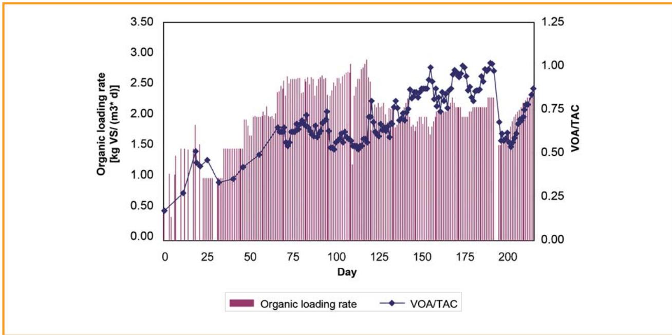
Figure 5.7: Progress of start-up phase of digester 1 with a deficiency of trace elements
