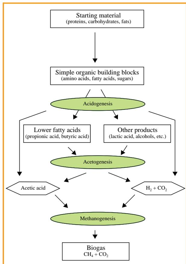
Figure 2.1: Schematic representation of anaerobic decomposition
