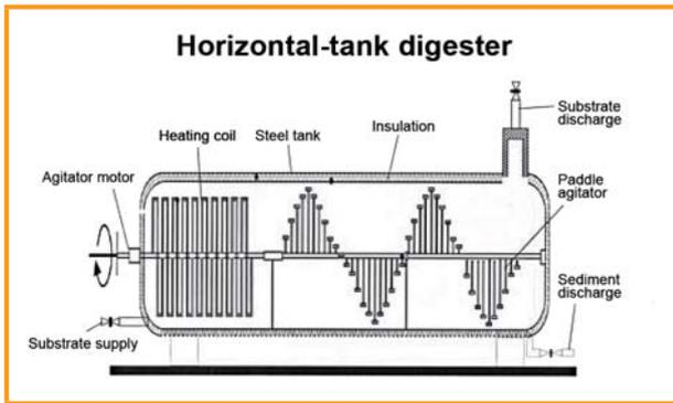
Figure 3.23: Plug-flow reactor (wet digestion) [3-4]
