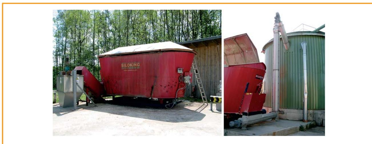
Figure 3.19: Feeding stackable biomass into the digester with screw conveyors [DBFZ]
