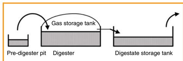
Figure 3.1: Schematic of the through-flow process
