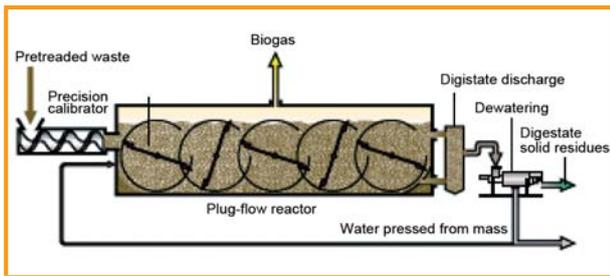
Figure 3.24: Plug-flow reactor (dry digestion) [Strabag-Umweltanlagen]
