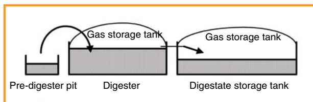
Figure 3.2: Schematic of the combination through-flow/buffer-tank process
