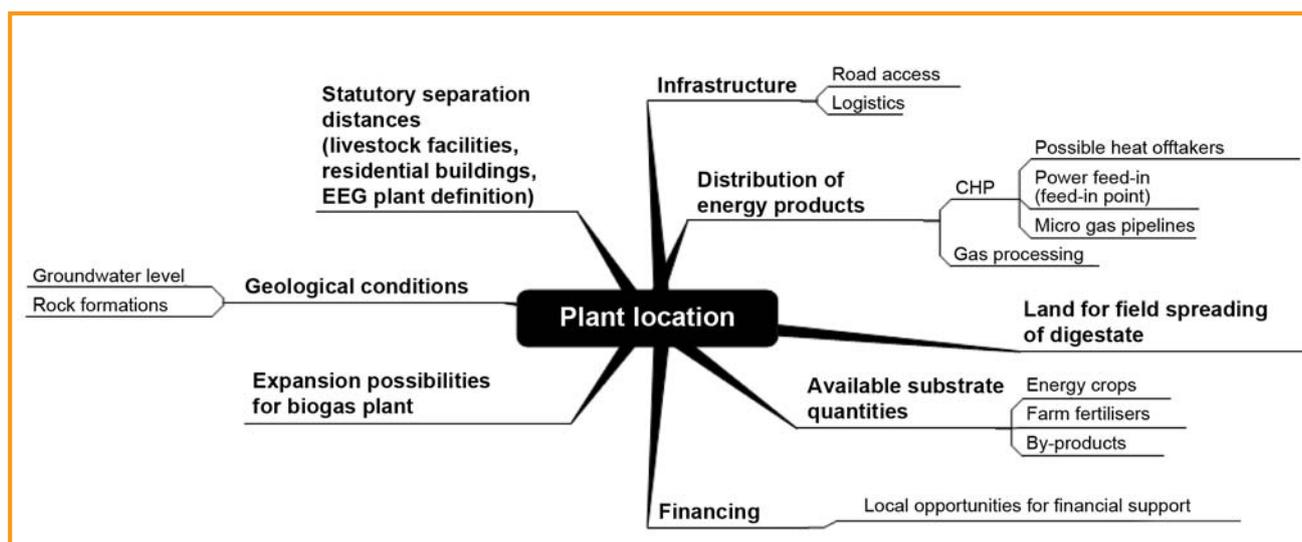
Figure 9.2: Parameters influencing the choice of plant location (CHP: combined heat and power)
