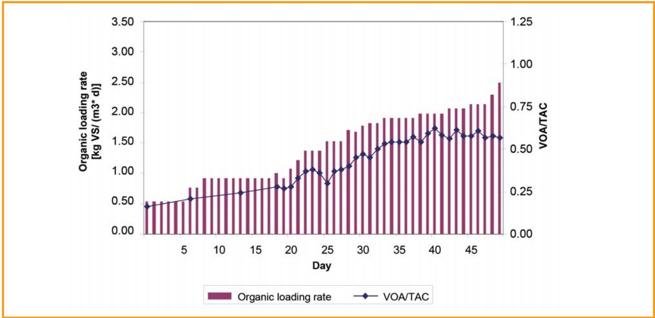
Figure 5.5: Progress of start-up phase, digester 2
