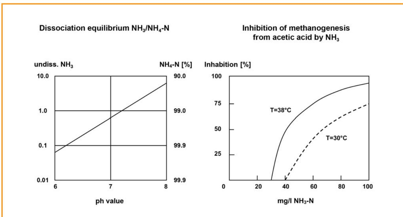
Figure 5.1: Inhibition of methanogenesis from acetic acid by  $NH_3$  (as per [5-2])
