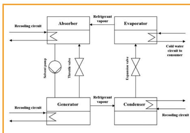
Figure 6.13: Functional diagram of an absorption refrigerator
