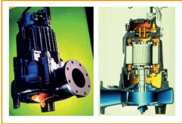
Figure 3.9: Submersible pump with cutting edges on the rotor as an example of a comminutor and pump combined in a single unit [ITT FLYGT Pumpen GmbH]
