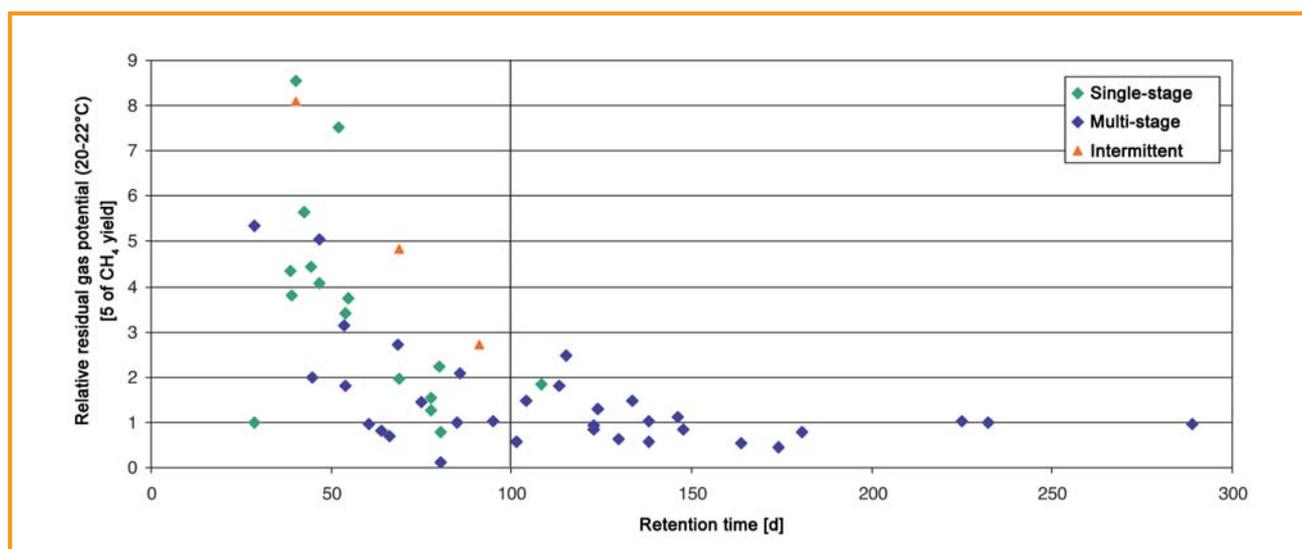
Figure 10.1: Correlation between relative residual gas potential at 20-22 °C and hydraulic retention time [10-8]
