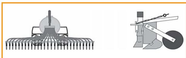
Figure 10.4: Cutting applicator
