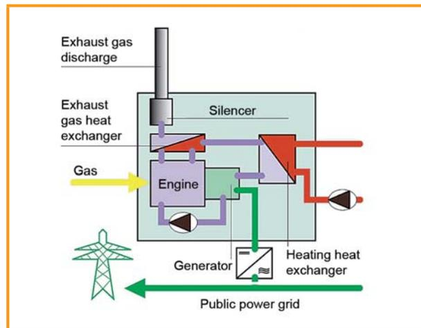
Figure 6.4: Schematic layout of a CHP unit [ASUE]
