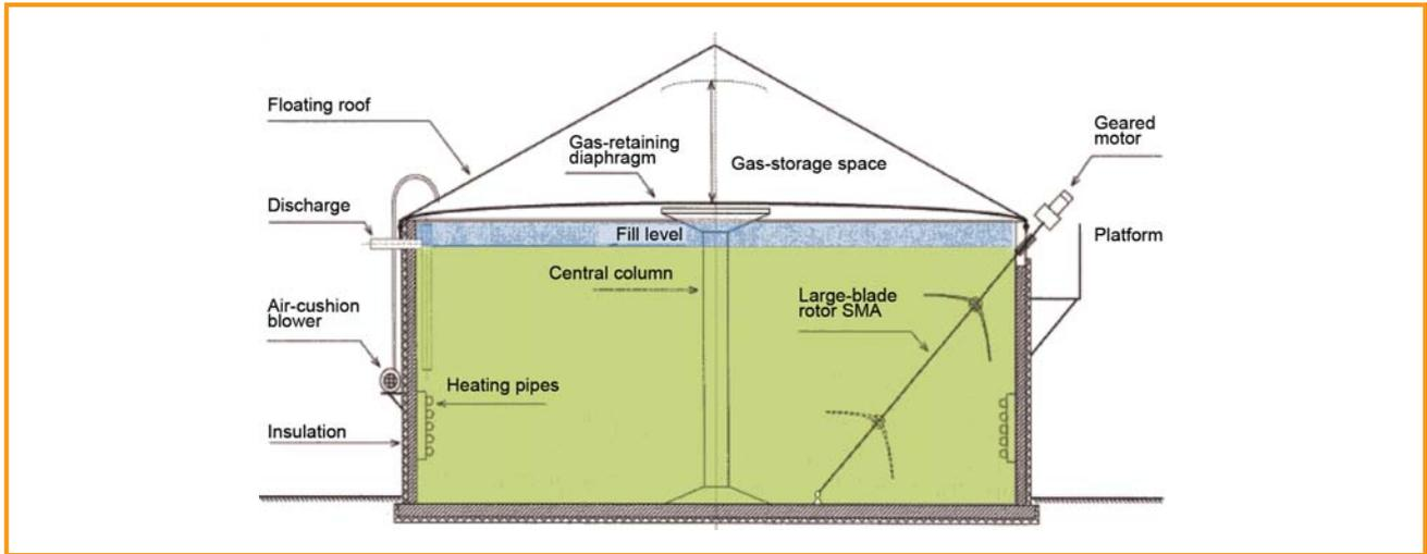
Figure 3.22: Stirred-tank reactor with long-shaft agitator and other internals [Anlagen- und Apparatebau Lütke GmbH]
