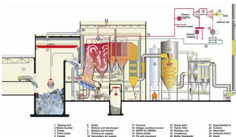
Figure 1 – Waste incineration process.
