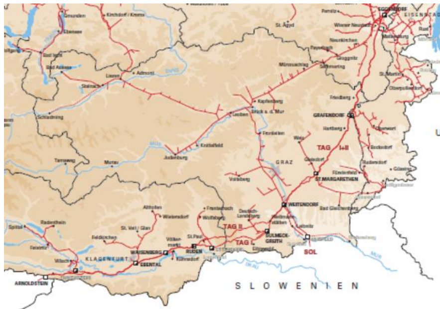
Figure 15: Gas grid in the south eastern part of Austria (Source: OMV)
