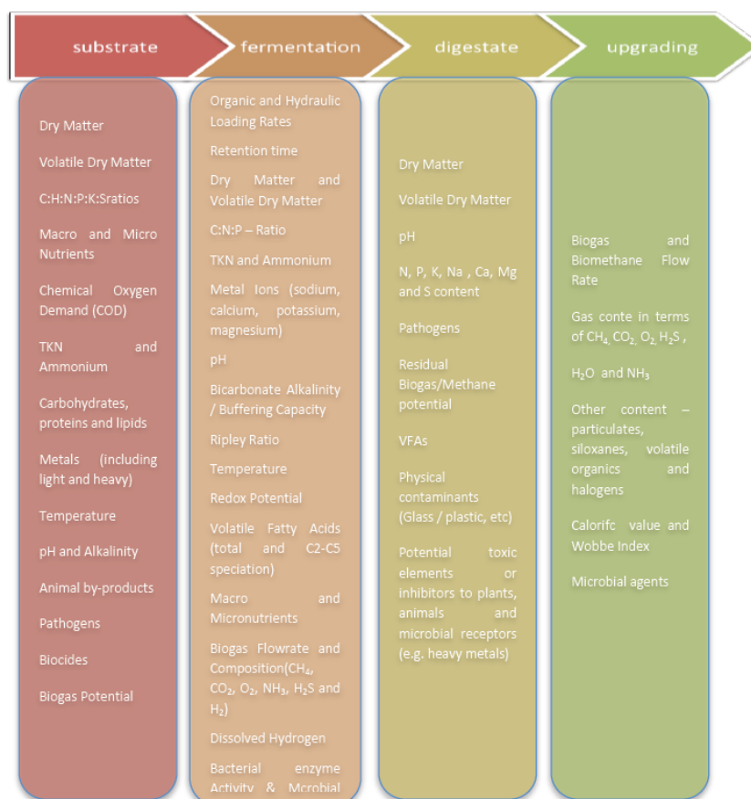
Figure 17: Monitoring parameters according to the phase of the anaerobic digestion (source: IEE Biomethane-Regions; D_5_1_Best_Practice_Monitoring (2012))
