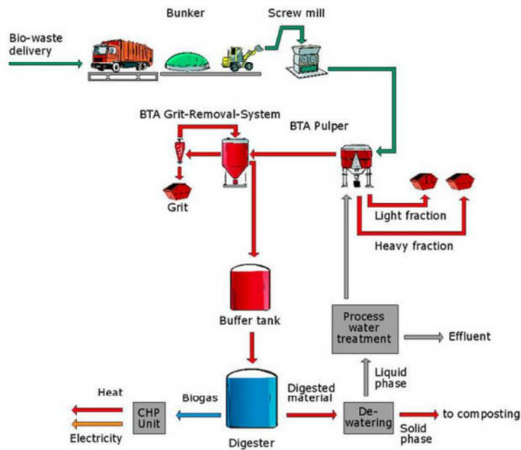
Figure 6: Schematic layout of BTA process
