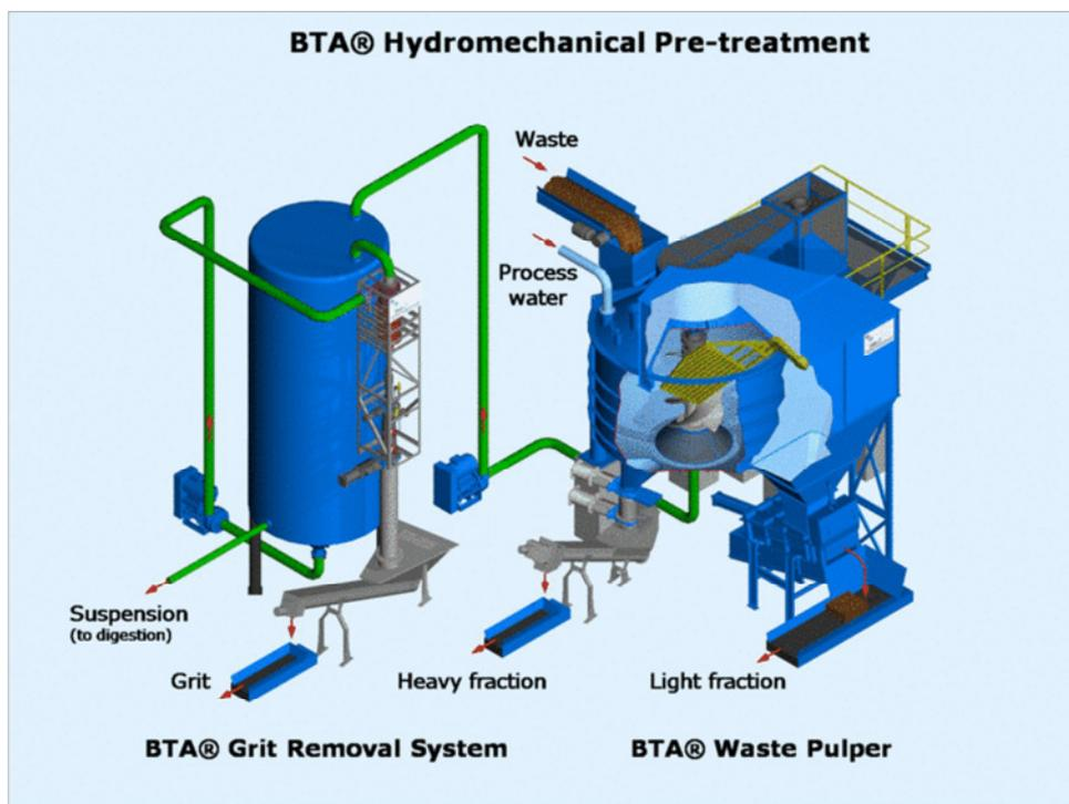
Figure 1: BTA Hydromechanical Pre-treatment
