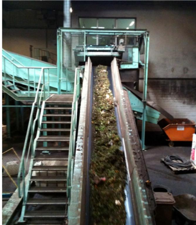
Figure 4: Biowaste transport
