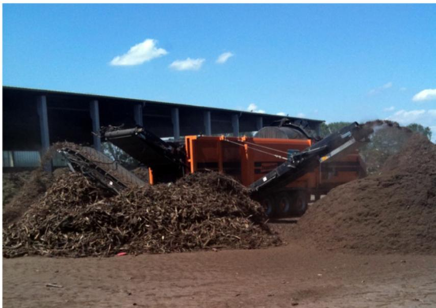
**Figure 19: Grinding and separation of biomass**
