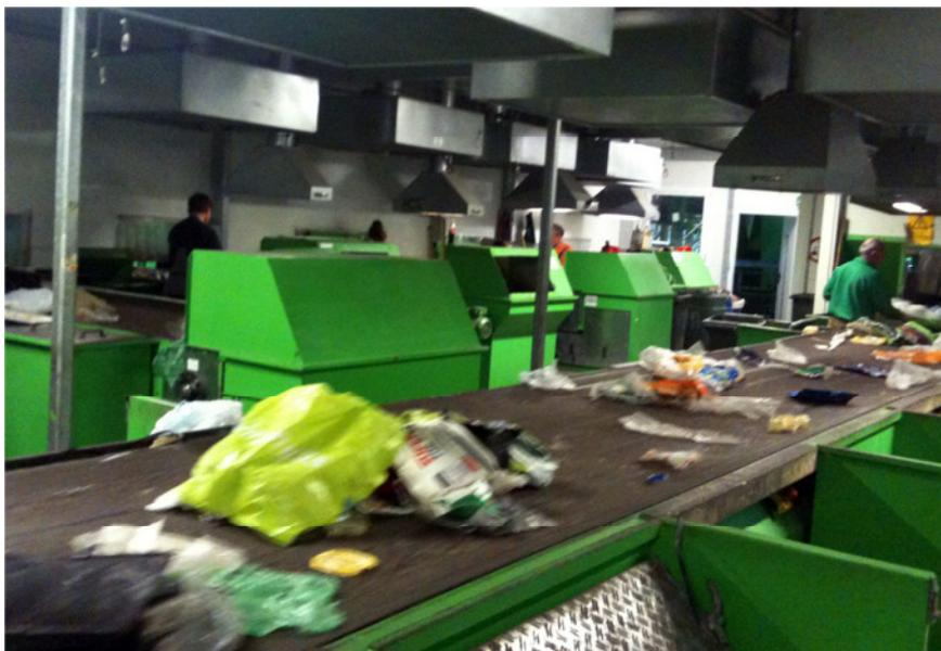
Figure 23: Manual separation
