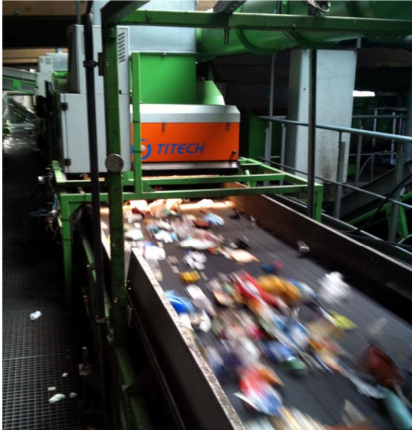
Figure 24: Automatic Separation of light fraction
