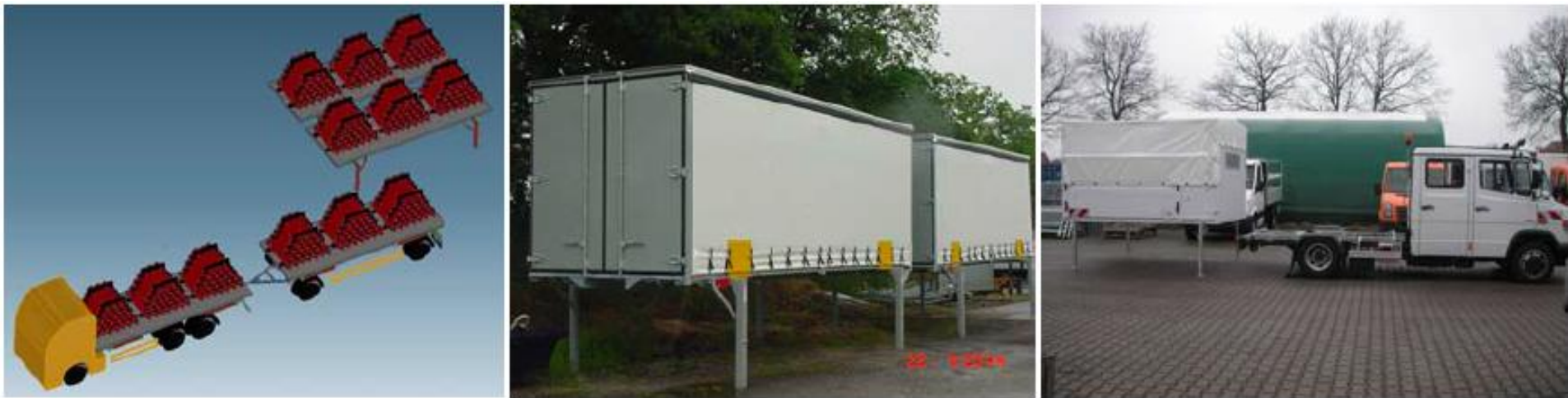
Figure 6: Pressurised gas tank transportation systems applying WAB system: design study of gas transportation truck with 150 cylinders of 80 litres volume for 220 bar (left); swap trailer system (mid); light lorry with swap trailer body (right); Source: Güssing Energy Technologies GmbH, Schoon Fahrzeugsysteme
