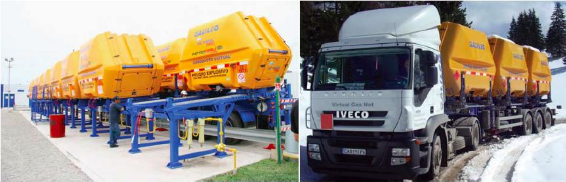
Figure 7: Pressurised gas transportation system – the Galileo system “virtual pipeline”; Source: Galileo SA
