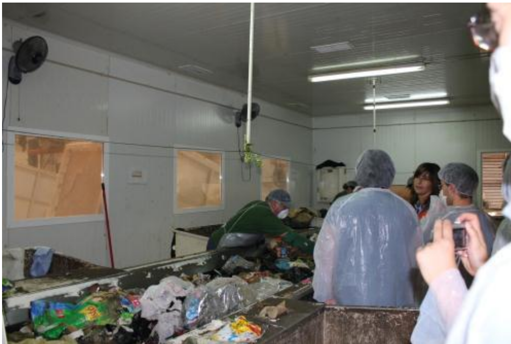
Figure 18 Visit to the solid waste treatment and upgrading integrated center. Manual separation line
