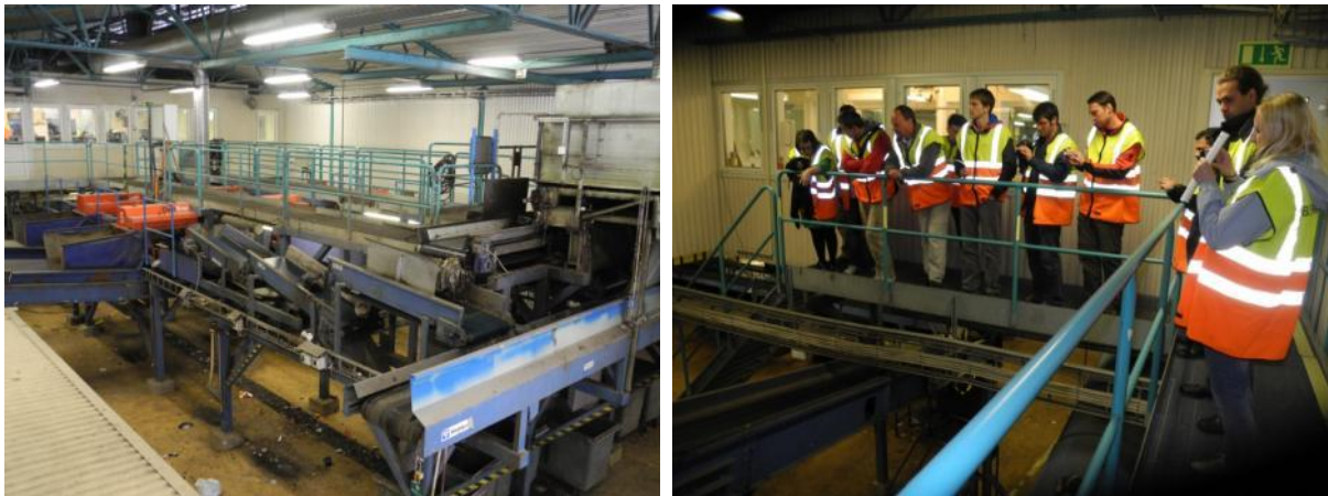
Picture 26: Separation process of incoming household waste by optical sensors
