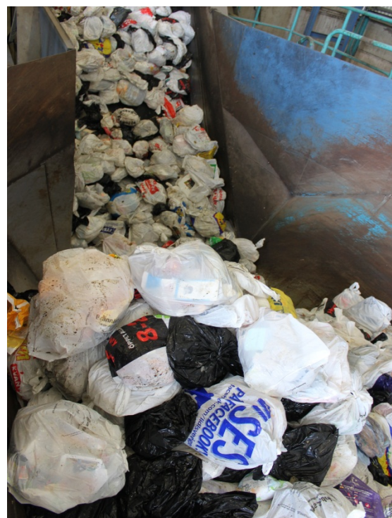
Figure 4: Example in Sweden: Mixed waste collection of bio-waste (black bags) and remaining MSW (white bags) which are sorted at the biogas facility
