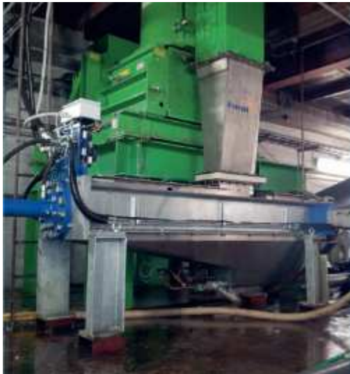
Figure 4-4 Example of separation press for smaller capacities (3 m 3 /h) of biowaste (source: Finsterwalder Umwelttechnik, www.fitec.com )
