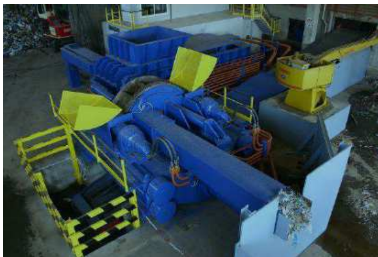
Figure 4-5 Example of press for mixed municipal waste (source: VMpress Technologies GmbH, http://www.vmpresstechnologies.com/ )
