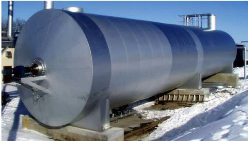
Figure 18 - Horizontal digester, built in Denmark (Nordish Folkecenter 2001). (Source: Biogas Handbook)
